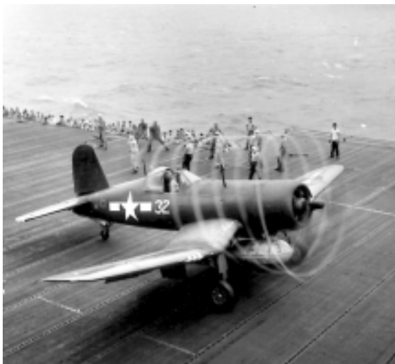
Vought Corsair propeller makes a corkscrew contrail in humid air. (Corbis)
